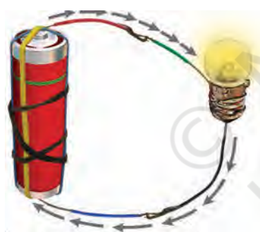
Fig.12.6 Direction of current in an electric circuit
