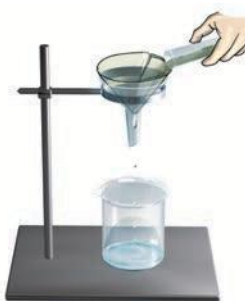
Fig. 5.10 Filtration using a filter paper
