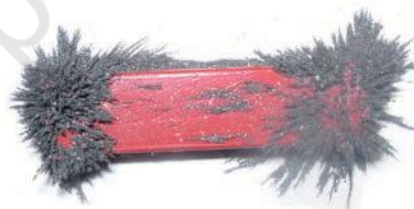
Fig. 13.7 Iron filings sticking to a bar magnet
