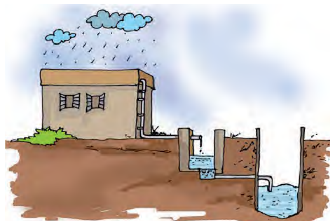
Fig. 14.13 Rooftop rainwater harvesting
