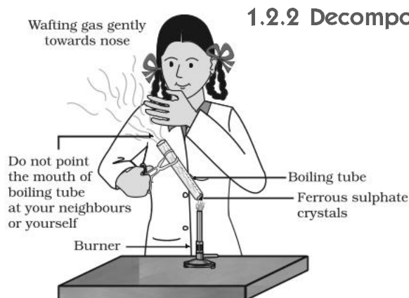
Figure 1.4 Correct way of heating the boiling tube containing crystals of ferrous sulphate and of smelling the odour
